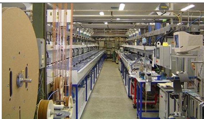
ציפוי אלקטרוליטי סליל לסליל. המקור: Interplex. Advanced Reel-to-Reel Plating Processes Improve Production Throughput, Quality and Costs. https://interplex.com/resources/technical-bulletins/plating/reel-to-reel-plating-improves-production-efficiency-and-saves-costs/
