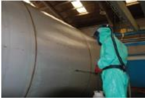
ניקוי בריסוס. המקור: Euro Inox. The European Stainless Steel Development Association. Post-fabrication Surface Treatment of Stainless Steel. 2015. https://www.edelstahl-rostoffrei.de/downloads/iser/PostFabricationSurfaceFinishing_EN.pdf
