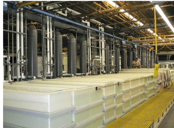
קו פוספטציה. המקור: Best Technology. Wash and Phosphate Pre-Treatment Conversion Coating Lines for Powder Coat Prep. https://www.besttechnologyinc.com/industrial-parts-washers-cleaning-systems/phosphate-lines-powder-coat-prep/
