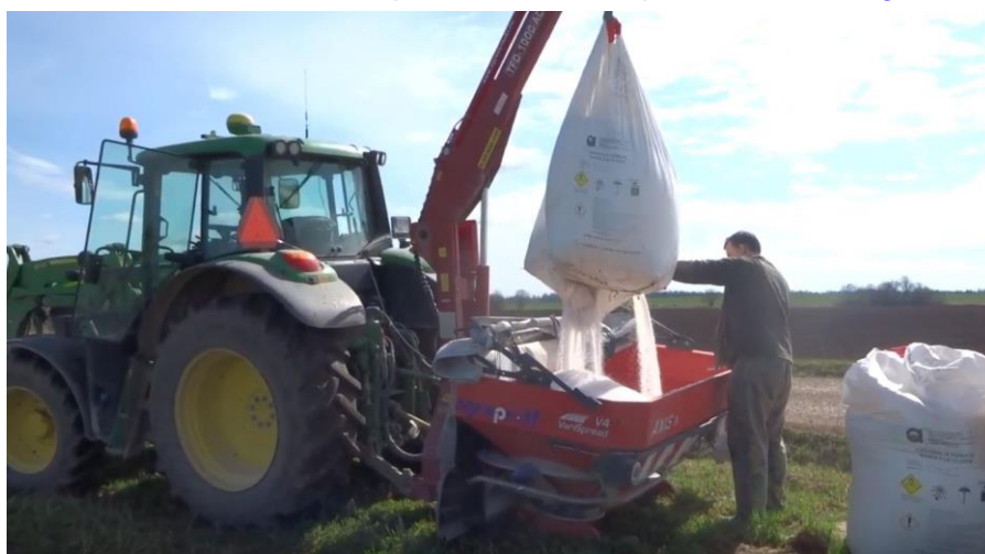
Farming 360. Rauch Axis-M 30.2 W fertilizer spreader loading with integrated crane. YouTube, 1 Jun, 2018. https://www.youtube.com/watch?v=3tNe27oLsxs
