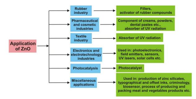
Zinc oxide is a unique material that exhibits semiconducting and piezoelectric dual properties, and has the broadest variety of nanostructures of all materials. These unique characteristics make it suitable for a wide variety of applications in optoelectronics, sensors, transducers, and the biomedical sciences [Kumar]. Nanoparticles of zinc oxide have the ability to absorb UV radiation, and are widely used in sun creams.
